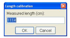
The window will show the length at the saw, measured by the machine (in this case 1588 mm) and it is waiting for the hand-measured length to be entered. When the hand-measured length has been measured, a new length factor will be calculated and this will be used on the logs cut from now on. The already cut logs will **not** be influenced by the new length calibration!
