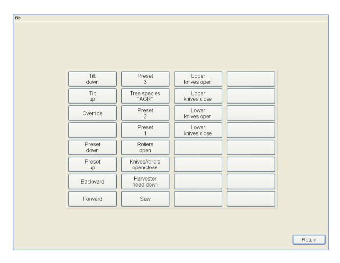
In this window you can choose, which function you want each button on the machine to have. By pushing a button on the machine, the button in question will marked in the window and by pushing the button in the window, the wanted function can be chosen from a list.
