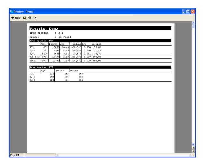
The printout is shown on white background. You can roll up and down in the printout with the scrollbar utmost to the right. In the menu line you have a number of symbols, which give some additional functions:
