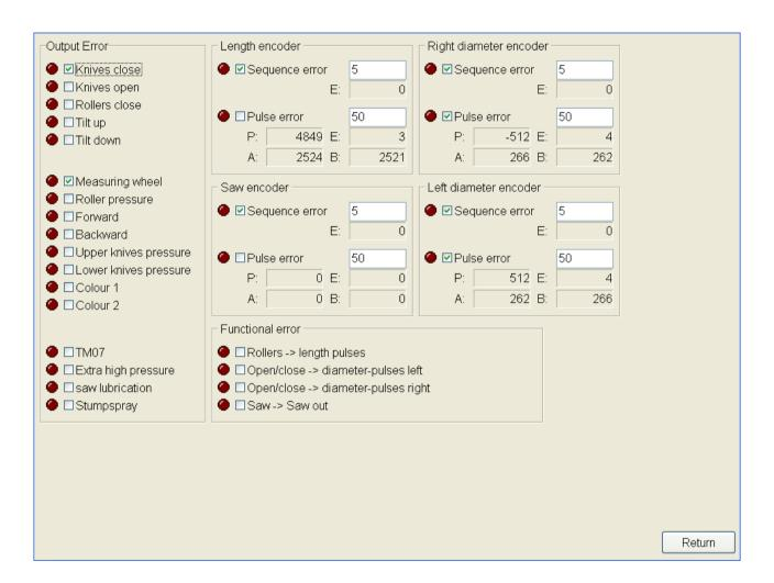
In this screen you can decide, which errors you want to be shown, if they should occur when using the machine. In order to activate a warning in case of error, the wanted error must be marked with a cross in the field against the error. For each encoder you can also indicate, how many of the different errors (sequential error and pulsations error) it shall take, before an error is shown.
