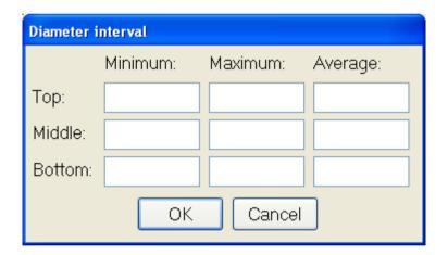
In this screen you must enter the relevant diameter demands for top, middle and bottom diameter respectively. You can enter demands for both minimum, maximum and average diameter. If you leave a field empty, this means that there is no demand regarding the combination in question, e.g. a value in "Minimum, Top", where all other fields are empty, will mean that the system will work according to one minimum top diameter only.
