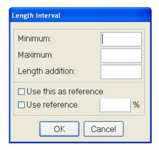
In this window you can enter the relevant length demands. If you leave out the minimum or the maximum, the system will work according to a maximum or a minimum demand only. If you want a certain length, you must enter this length in both the minimum and the maximum field.
