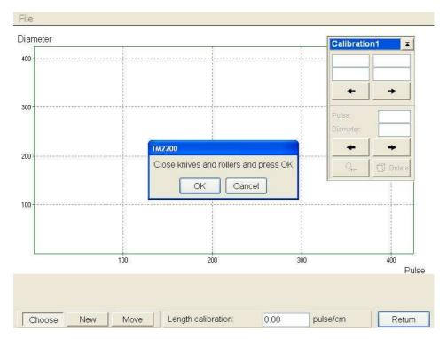
As you see it only has two points, the full open diameter and the full closed diameter. The vertical scale on the left hand side is the diameter, and the horizontal scale at the bottom is the pulses coming from the diameter encoder(s)
