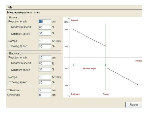
If you leave the maneuver pattern box blank and then instead press "New maneuver pattern" you can make your own from scratch. Insert a name, press "OK" and insert values at the left side. You will see the graph be drawn according to your entered values. Notice! Tolerance is the "cutting window" in which the system will stop and accept the length. E.g. if the preset say 500 cm. + 10 cm. the "cutting window" will be from 510 cm to 513 cm.
