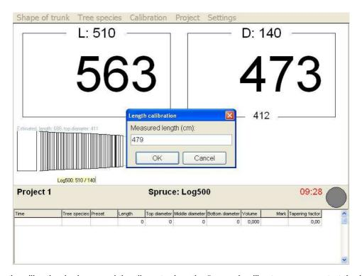
Now the length calibration is done, and the diameter has the "ground calibrator can now start the job. Remember to do control measuring occasionally. The most important control measurings are at the start of a new project.
