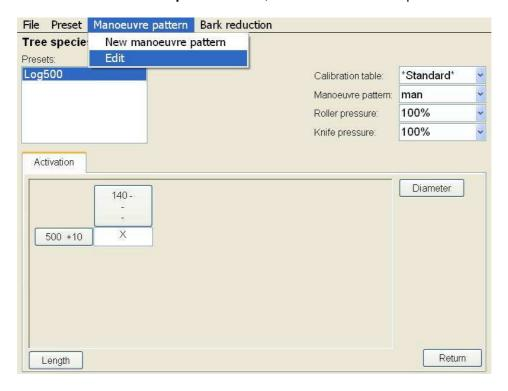
Maneuver pattern are settings for how the feeding rollers work. To the left are the editable settings, and on the graph at the right hade-side you see the settings graphically. Try to change a value in a box and watch the graph.
