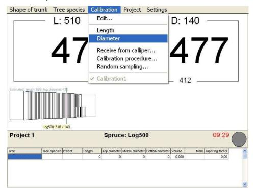
Enter the measured diameter in the message box and press "OK". You will see the diameter now changes on the screen.
