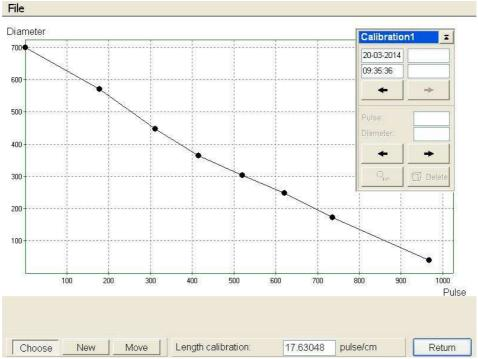
It might look like this; the point (the square) has the same (or lower diameter) as the next point. You can release the next point from the calibration (see Chapter xx) with  $\mathbf{O}_{+/}$  and see if the new point is closer to the line.
