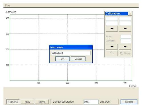
The message box tells you to close knife and rollers. When you see the knives and rollers are fully closed, you press "**OK**" and the new diameter calibration is made.
