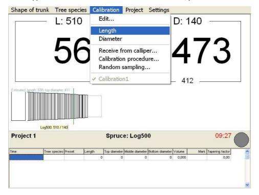
In the message box, you now enter the measured length and press the "OK" button. Watch the length that now has changed to the length you entered. (Notice! Due to calculation, the length can vary + -1 cm.)
