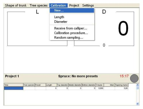
You are now in the Calibration window. Type a name to your new calibration and press "**OK**". <u>Before you press the "**OK**" button make sure the head is fully opened.</u>
